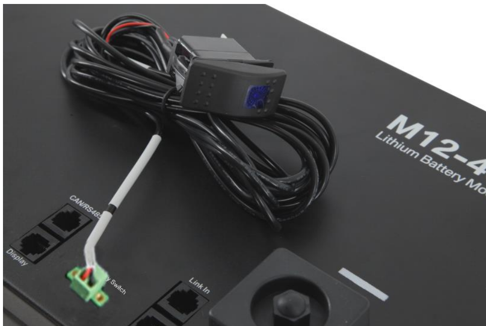
Figure 2-11 Schematic diagram of battery switch installation and wiring
