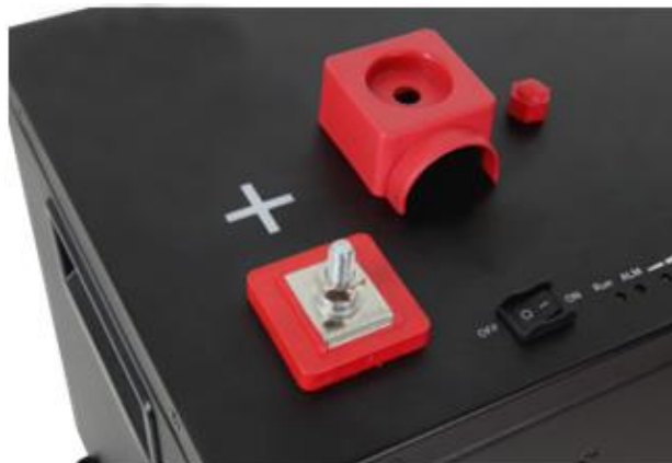
Figure 2-7 Remove the protective cover of the lithium battery
